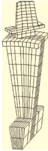
Fig. 6 Finite element model of bladed disk sector
