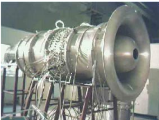
Fig. 1 Side view of compressor test rig
